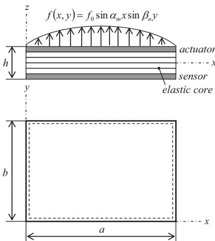
Fig. 1. Smart laminate configuration.
