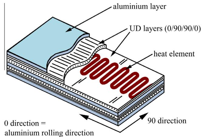
Fig. 1. Schematic lay-up of a heated GLARE laminate.
