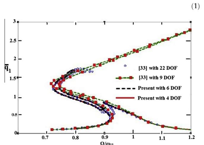
**Fig. 2.** MCM<sub>1</sub> of shell of simply supported movable edges  $a = b = 0.1$  m,  $h = 0.001$  m,  $R_x = R_y = 1$  m,  $E = 206$  GPa,  $\nu = 0.3$ ,  $\rho = 7800$  kg/m<sup>3</sup>,  $\hat{f} = 31.2$  N, and  $\zeta = 0.004$ .
