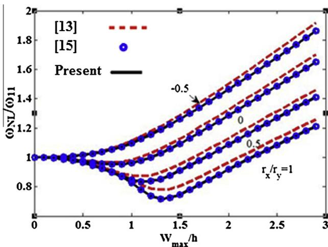
**Fig. 1.** Nonlinear free vibration of isotropic simply supported shallow shell with movable edges  $r_x = \frac{R_x}{a}, r_y = \frac{R_y}{b}, E = 70$  GPa,  $\nu = 0.3$ , and  $\rho = 2702$  kg/m<sup>3</sup>.
