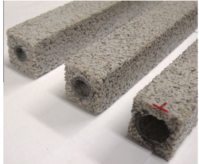
Fig. 1. Polymer concretes embedding PMMA pipes.
