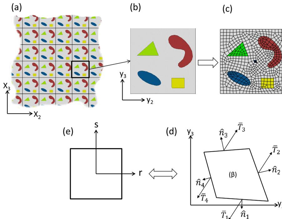
**Fig. 1.** Schematic representation of doubly periodic material at the composite and subcell level. For a given periodic composite material (a), a RUC can be identified and isolated (b). Subfigure (c) shows a RUC divided into subcells. The mapping of subcell from the physical to the parametrical coordinate system is illustrated in subfigure (d) and (e).  $\bar{T}_i$  and  $\hat{n}_i$  are the traction applied on face  $i$  and its normal vector, respectively.
