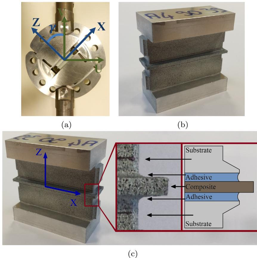
**Fig. 1.** Principle of the Arcan test (a). Specimen used to test the out-of-plane properties of the composite (b). Detail of the substrate design to reduce the stress concentrations close to the free edge (c).
