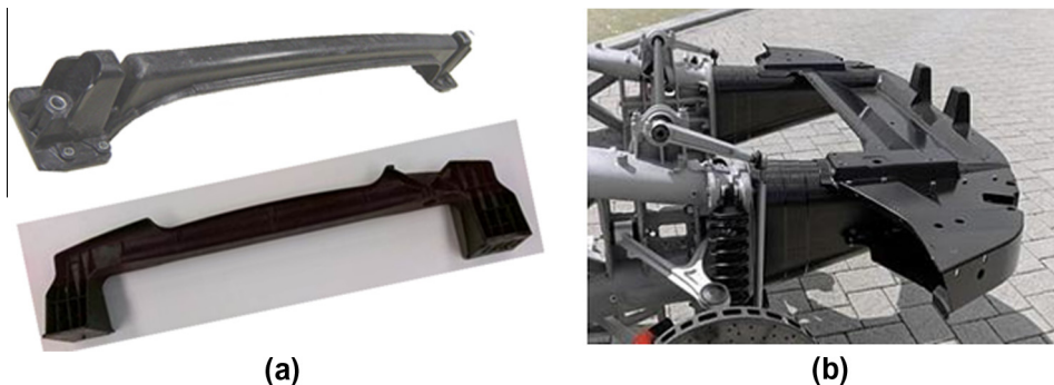
Fig. 1. Integrated composite solution developed by Quadrant Plastic Composites International (a) and used on Mercedes for top class vehicle (b).
