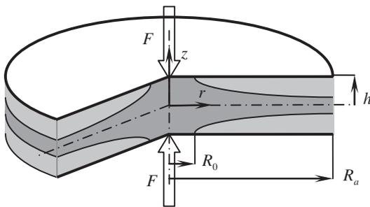
Fig. 1. Schematic diagram of the squeeze flow between two parallel disks (dark region is the core of the fluid with high viscosity).
