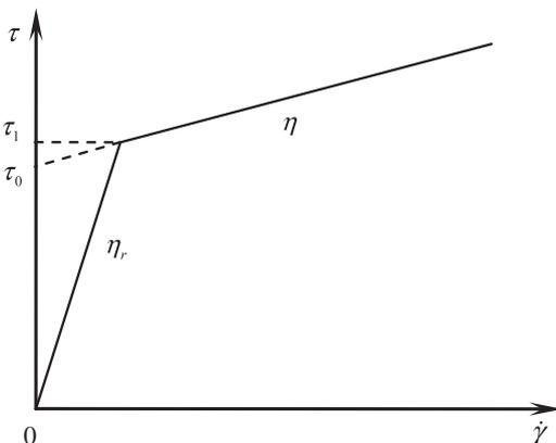
Fig. 2. Model for the biviscous fluid.
