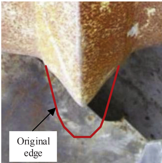
Fig. 1. Field observation of lateral continuous wear on disc cutter ring [39].
