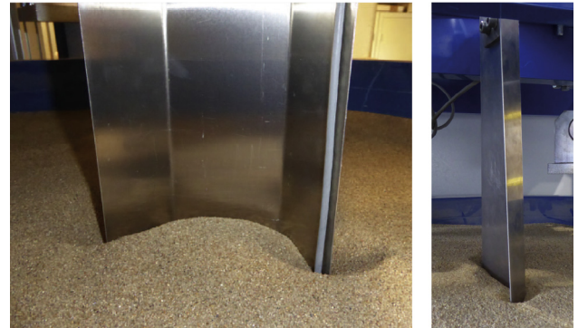
Fig. 4. Appearance of hoppers at soil surface due to jacking of U-section (left) and Z-section (right).
