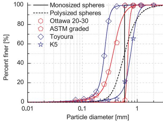
Fig. 1. Grain size distribution curves of granular assemblies used in this study. Symbols are fitted by Fredlund et al. [45].
