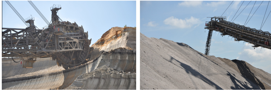
Fig. 1. Excavation of the soil layers (left) and deposition of the mixed clays (right) in the open-pit mining.
