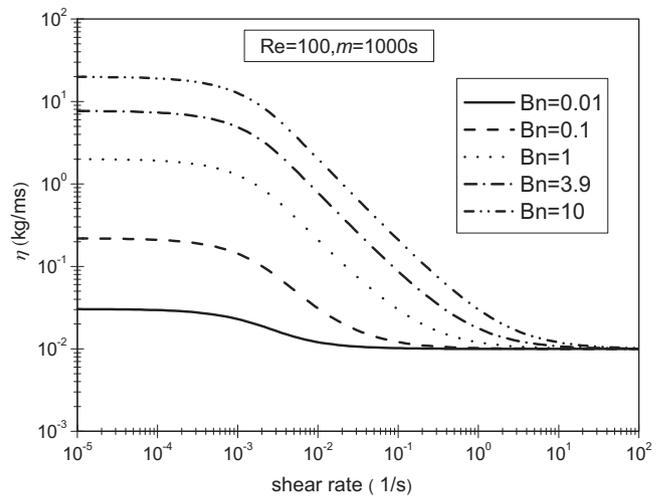
**Fig. 2.** The Bingham apparent viscosity against shear rate  $\dot{\gamma}$  for different Bingham numbers at  $Re = 100$  and  $m = 1000$  s.
