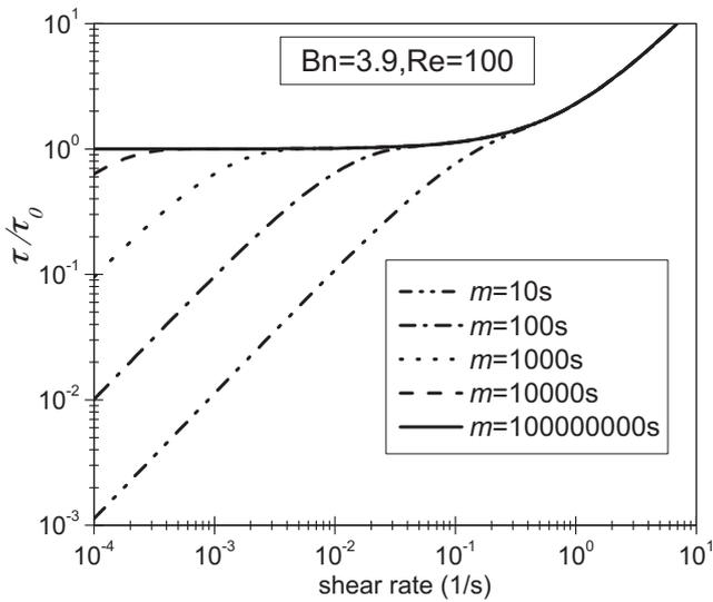
**Fig. 1.** The dimensionless shear stress against shear rate  $\dot{\gamma}$  according to the modified Bingham constitutive equation (2) for several values of the exponent  $m$ .
