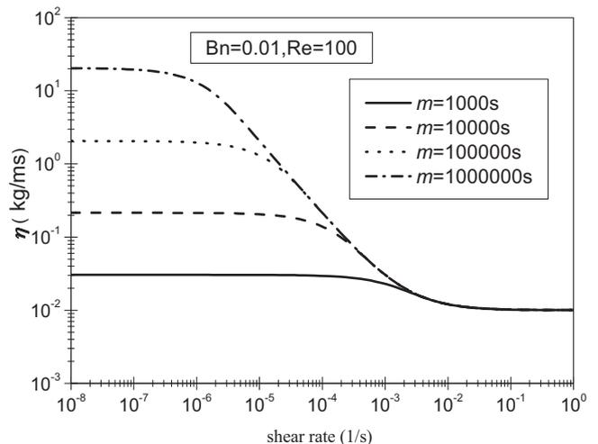
**Fig. 3.** The Bingham apparent viscosity against shear rate  $\dot{\gamma}$  for different values of exponent  $m$  at a small Bingham number  $Bn = 0.01$  and  $Re = 100$ .
