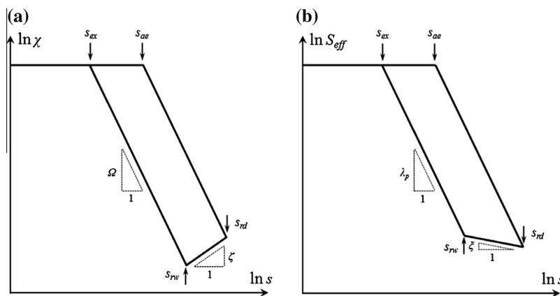
**Fig. 1.** (a) Evolution of effective stress parameter and (b) soil water characteristic curve including hydraulic hysteresis.
