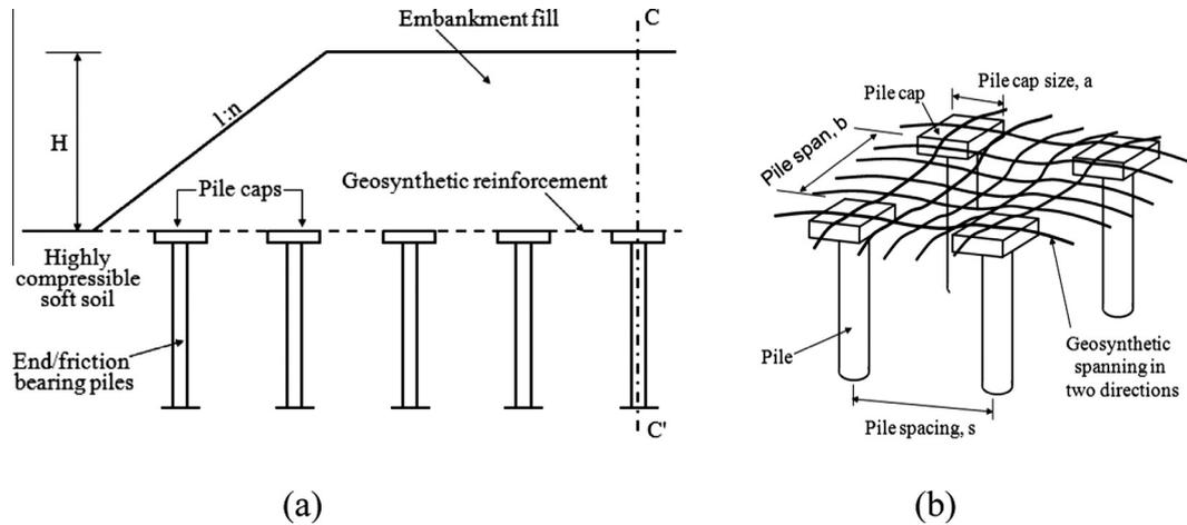
Fig. 1. (a) A section of a piled embankment and (b) the general layout of piles (caps) and reinforcements (after Kempton et al. [20]).
