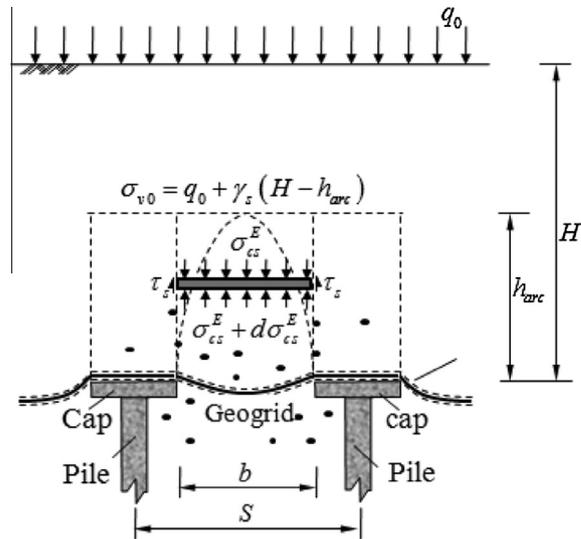
Fig. 2. Load transfer mechanisms of GRPS embankments and the arching effect.
