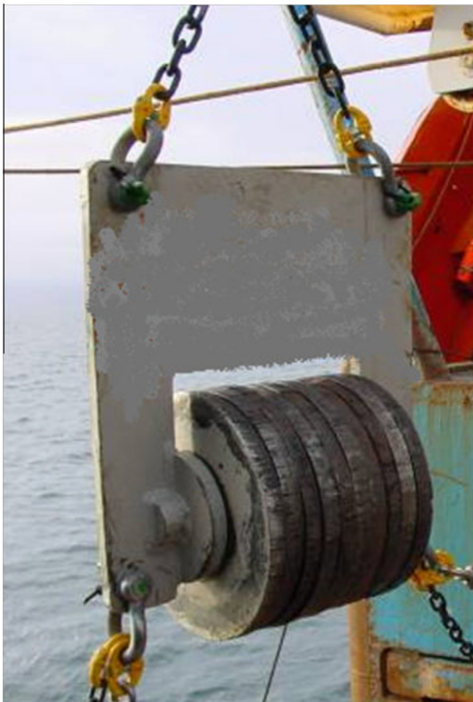
Fig. 2. Example of a clump weight used with twin trawls.
