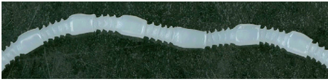
Fig. 1. Stick-slip defect of a metalocene polyethylene (mPE). Sharkskined zones correspond to branch I, smooth ones to branch II.
