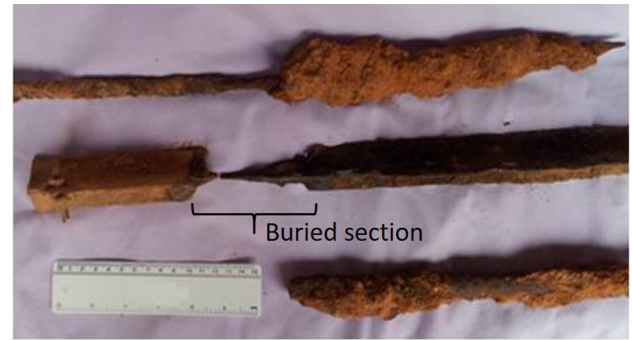
Fig. 1. Corroded reinforcement from 30-year-old CSRE wall.
