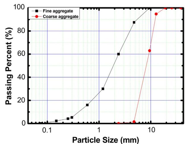
Fig. 1. Particle size distribution of fine and coarse aggregates.
