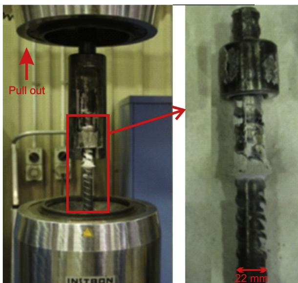
Fig. 1. Debonding failure of a mortar-bolt interface subjected to axial loading. Adapted from [15].
