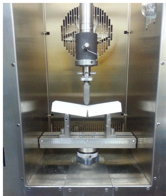
Fig. 1. The device for the three-point bending test inside the oven.
