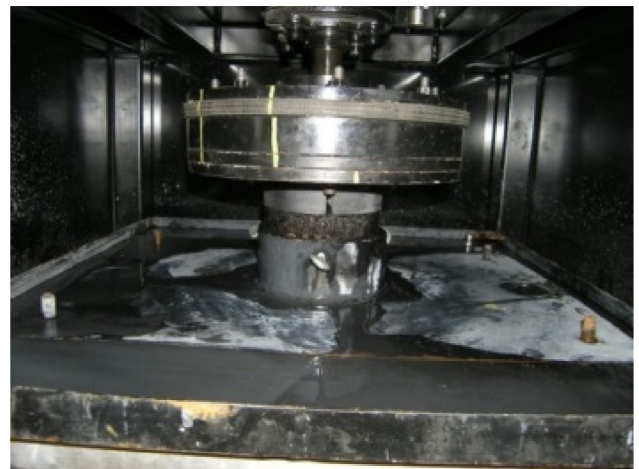
(b) Close-up of the rubber shoe-specimen interface
