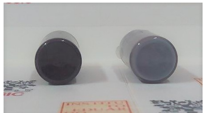
Fig. 1. Aspect of the reversibly thermochromic slurry at a temperature lower (left, at 8 ^{\circ}\text{C} ) and higher (right, at 50 ^{\circ}\text{C} ) than the transition temperature of 31 ^{\circ}\text{C} .
