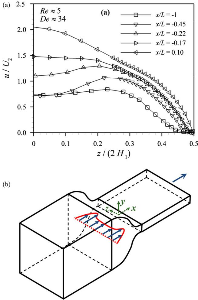
**Fig. 1.** (a) Spanwise profiles of the streamwise velocity for an aqueous solution of 3000 ppm polyacrylamide in an 8:1 planar gradual contraction flow  $Re \approx 5$ ,  $De \approx 34$  (adapted from Ref. [3]) and (b) schematic of the geometry and coordinate axis.
