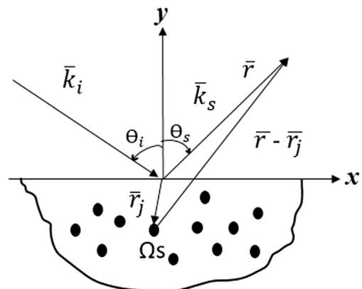
Fig. 1. Scattering of a domain with  $N$  scattering points.
