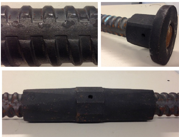
Fig. 1. Details of threaded bar and grout-filled end-anchorage device and splice sleeve.
