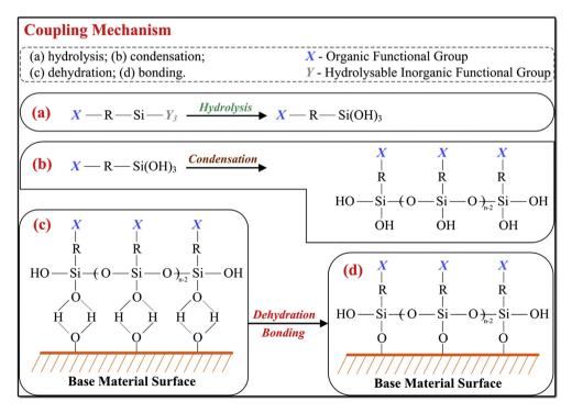
Fig. 1. Coupling mechanisms of common silane coupling agent.
