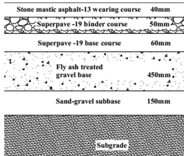
Fig. 1. Pavement structure for the field test section.
