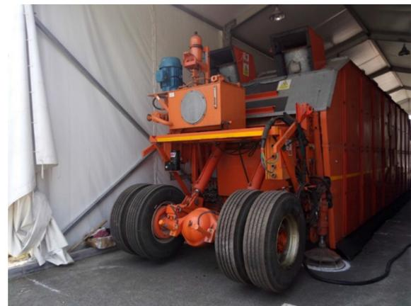
Fig. 2. The MLS66 machine at the field test section.
