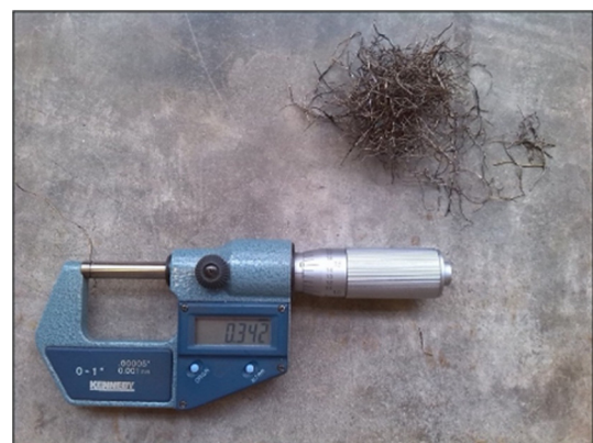
Fig. 2. Recycled steel fiber appearance and diameter measurement process.
