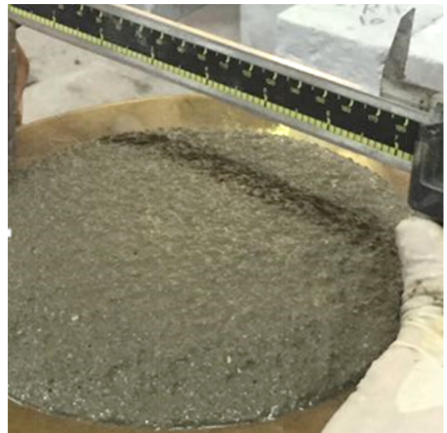
Fig. 3. Measurement of flow spread diameter.
