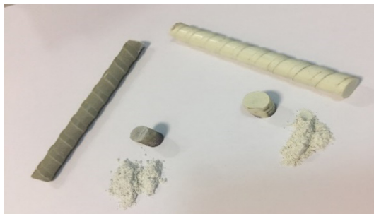
Fig. 1. GFRP bars used in the current study.
