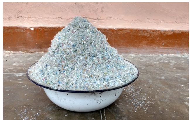
Fig. 3. Plastic waste for fine aggregate replacement.
