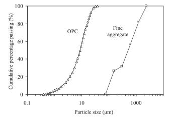
Fig. 1. Particle size distributions of OPC and fine aggregate.
