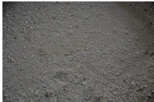
Fig. 1. Fine bone china ceramic aggregate.
