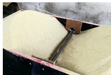
Fig. 1. Test setup of dry sand simulation tank and example of the lap splice in dry sand (unit: mm).
