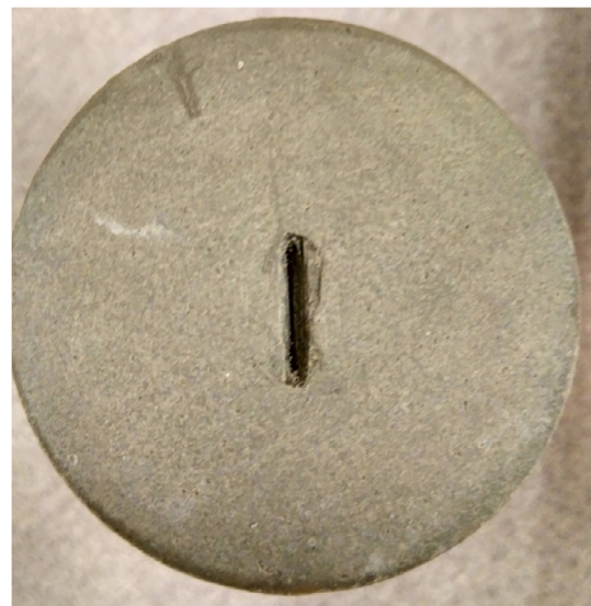
Fig. 2. Specimen with cut slot after curing.
