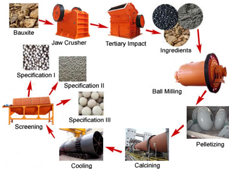
Fig. 1. The flowchart of LECA production ( http://www.ftmmachinery.com ).
