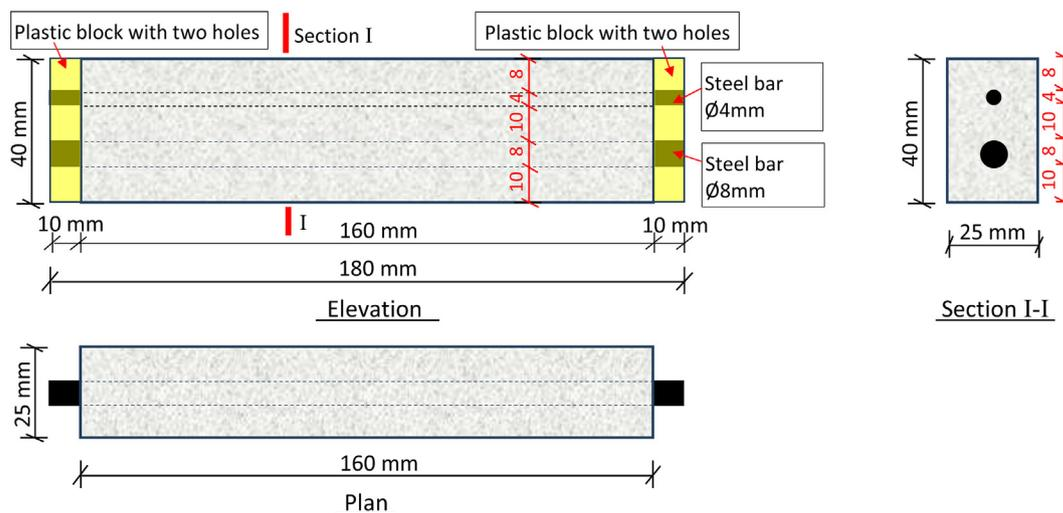
Fig. 1. The shape and size of the prismatic specimens used in this project and the positions of the steel reinforcements embedded in the specimens.
