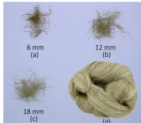
Fig. 3. (a) Hemp fiber in 6 mm length, (b) Hemp fiber in 12 mm length, (c) Hemp fiber in 18 mm length (d) Carded hemp fiber.
