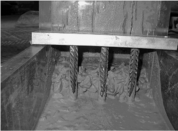
Fig. 1. Granular blocking within the flow duration of SCC (from [1]).
