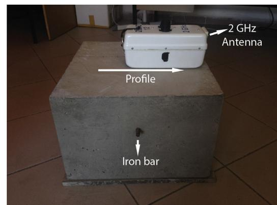
Fig. 2. C-30 concrete sample, 2 GHz GPR antenna and the profile direction.
