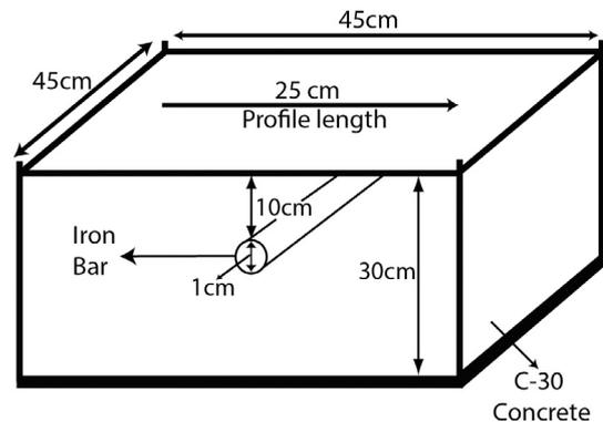
Fig. 1. The sizes of experimental model.
