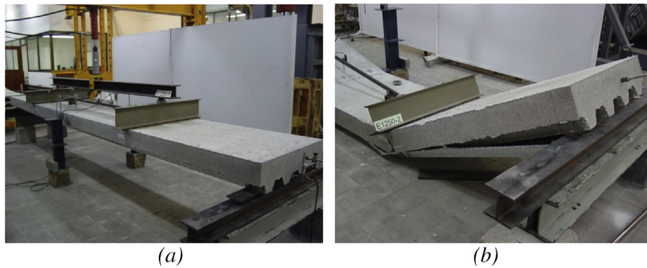
Fig. 2. a) Standard bending test set-up; b) Longitudinal slip failure and vertical detachment.
