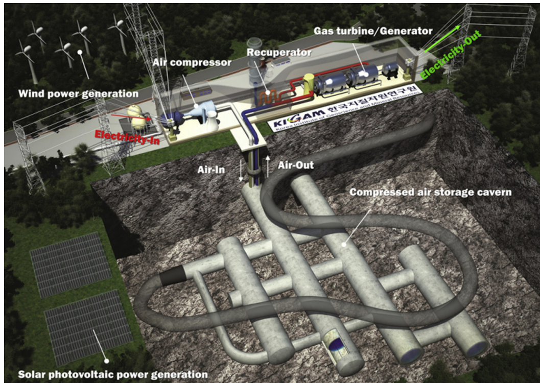
Fig. 1. Diagram of a compressed air energy storage plant using underground lined rock caverns, from Ref. [6].
