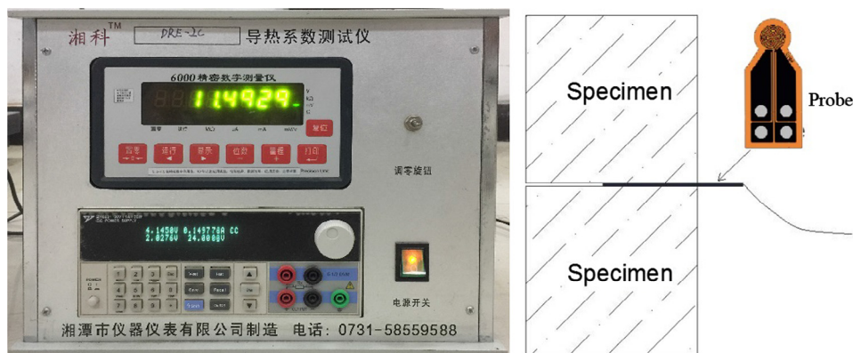
Fig. 2. DRE-2C thermal conductivity tester and probe placement.
