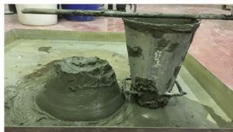
(c) Typical slump test
