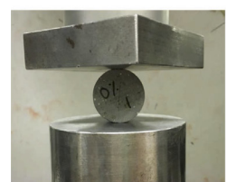
(e) Typical split test
