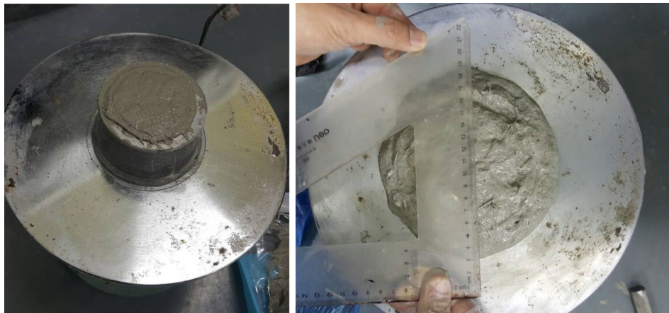
Fig. 1. Fluidity test of MOC-ECC.
