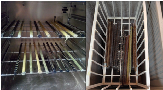
Fig. 3. Heated and cooled FRP bars.
