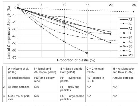
Fig. 1. The relationship between plastic replacement and loss in compressive strength.
