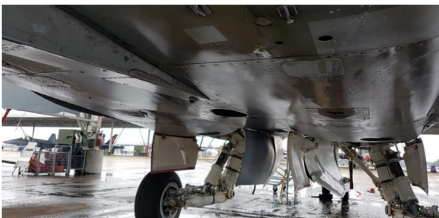
Fig. 1. Underbelly of an F/A-18 with APU featured in the centre of the photo [3].
