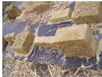
(a) Brick with fibres ( 1\ 200 \text{ kg}\cdot\text{m}^{-3} ).
